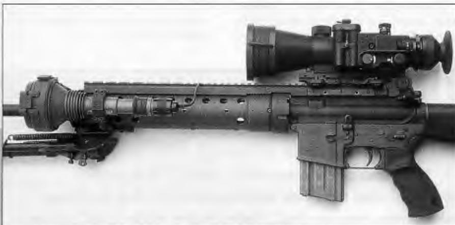
With the 4X Raptor, an M3 SureFire Tactical Light with an infrared (IR) filter was mounted on the fore-end using an A.R.M.S. #22 ThrowLever ring. Invisible to the naked eye, this powerful light increased the brightness seen through the Raptor by about 400%. A Harris Bipod was mounted on the bottom M1913 rail.
